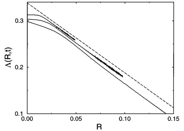
FIG. 2. The finite-time comoving Lyapunov exponents  $\Lambda(R, t)$  as a function of rate  $R$  at time  $t = 20, 40$ , and  $80$  (from bottom to top), for coupled tent maps with  $\alpha = \frac{3}{2}$ ,  $L = 5001$ , and  $\varepsilon = \frac{1}{3}$ . The dashed line represents the asymptotic expression  $\Lambda(R) = \lambda - \frac{3}{2}R$ .
