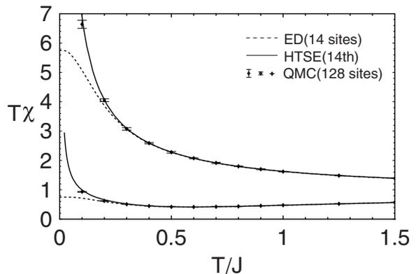
Fig. 2. Temperature times susceptibility per unit cell for the MS chain with  $s = 1/2$  and  $S = 1$ , calculated by HTSE, QMC, and ED.
