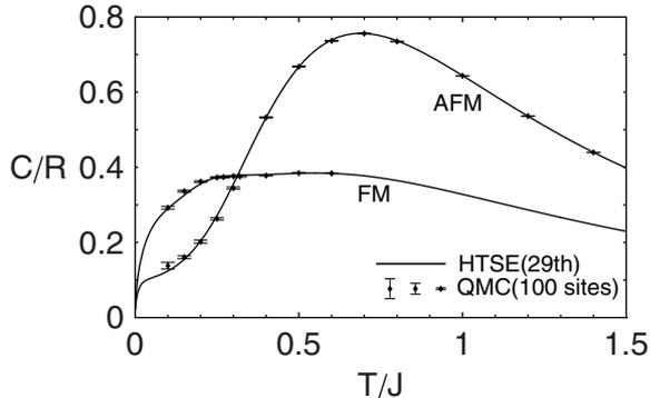
Fig. 1. The specific heat per unit cell for the MS chain with  $s = 1/2$  and  $S = 1$ , calculated by HTSE and QMC.
